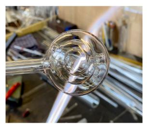
nuclear bulb is made of three layers of spherical glass, each of which is connected to a pair of electrodes. Imagine the atmosphere where air become thinner at higher altitude, the sky would appear a transition from bright to dark.
